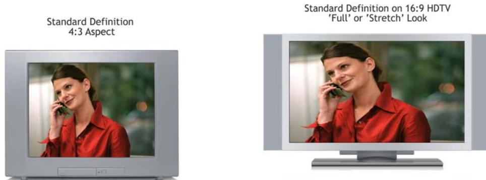
Figure 17: SD on 4:3 Monitor and 16:9 Monitor in 'Full' mode
