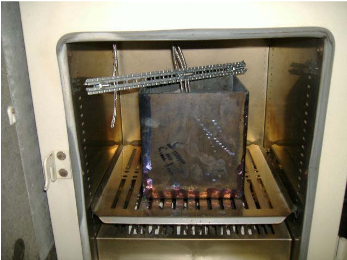
Figure 3. Laboratory Setup for Auto-Ignition Tests.
