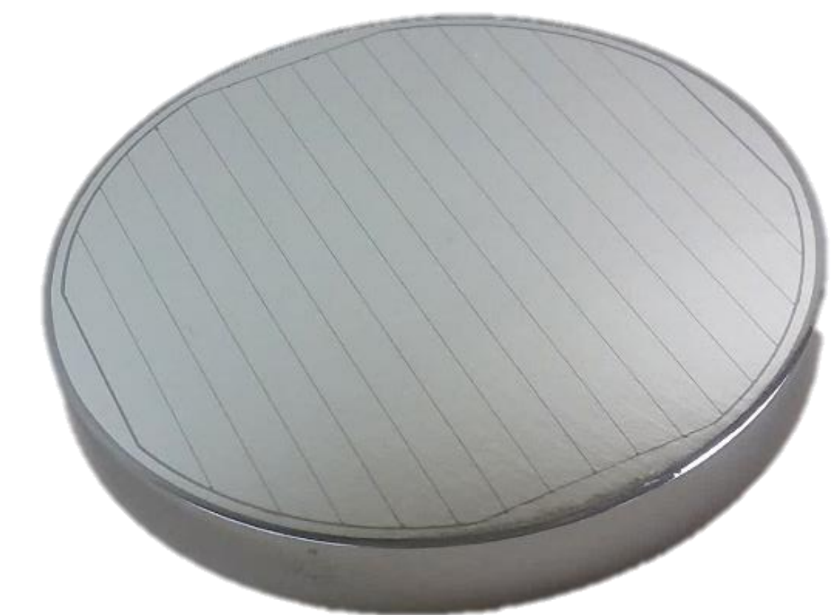
The GeGI detector crystal. There are 16 strips orthogonally on the front and back faces.
