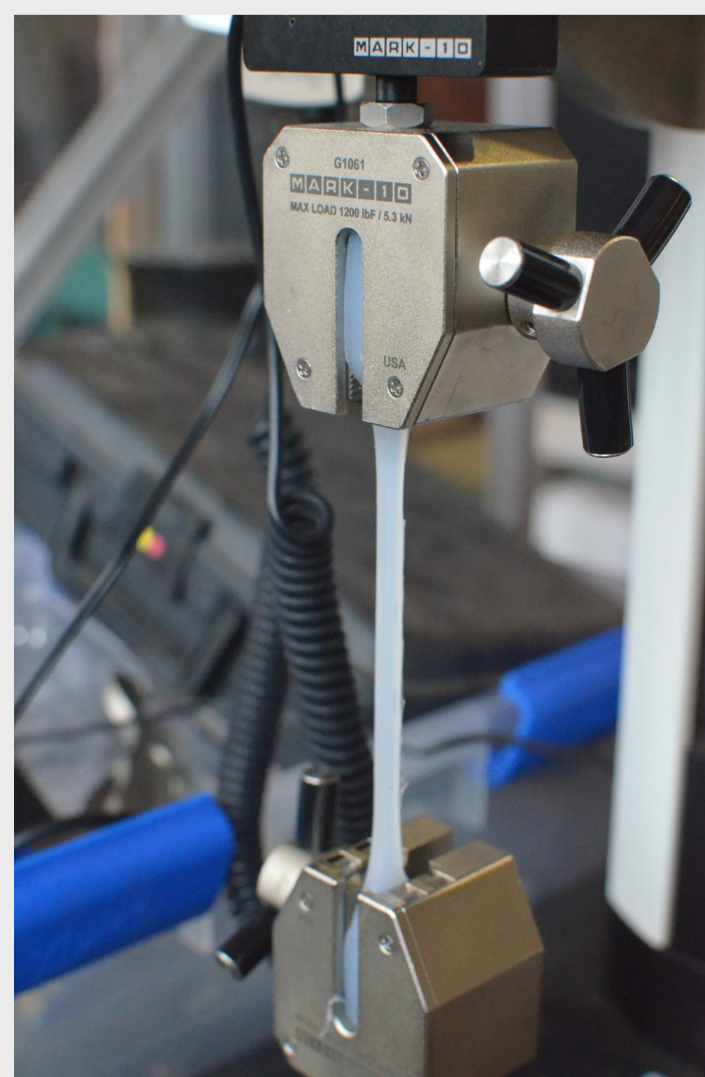
Figure 4. A dogbone sample undergoing elongation and tensile strength testing in the Mark 10 machine.
