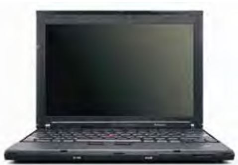
Lightweight magnesium alloy optimizes the Lenovo X201 laptop and X201 tablet's toughness and portability for today's mobile workforce. © Photos courtesy of Lenovo. Used with permission.
