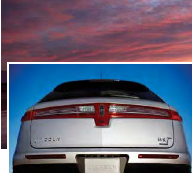
The Lincoln MKT liftgate design uses magnesium and aluminum panels to create a liftgate that is 40 percent lighter than a standard steel liftgate. © Photos courtesy of Ford Motor Company. Used with permission.
