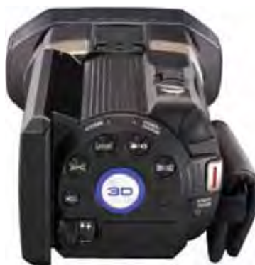
Weighing just 1.4 pounds (590 grams) with the battery, this JVC magnesium frame video camera uses two lenses and two 3.32 mega pixel CMOS sensors to capture full HD 3D video by processing left and right images simultaneously using a high-speed imaging engine. © Photos courtesy of JVC USA. Used with permission.
