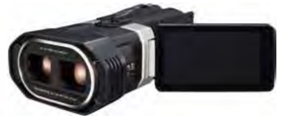
Weighing just 1.4 pounds (590 grams) with the battery, this JVC magnesium frame video camera uses two lenses and two 3.32 mega pixel CMOS sensors to capture full HD 3D video by processing left and right images simultaneously using a high-speed imaging engine. © Photos courtesy of JVC USA. Used with permission.
