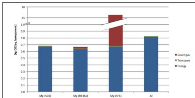
Figure 3. Contribution of cover gas, energy, and transport to the GHG emissions from the die casting process.
