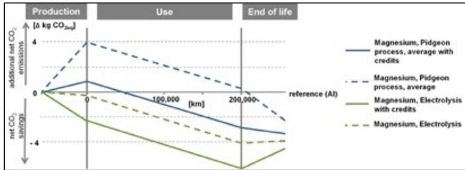
Figure 4. Net difference of GHG emissions of the magnesium steering wheel frame compared to the aluminum alternative.
