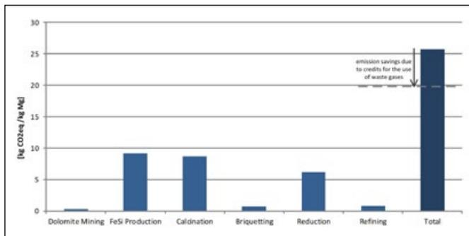
Figure 1. GHG emissions from the Pidgeon process.
