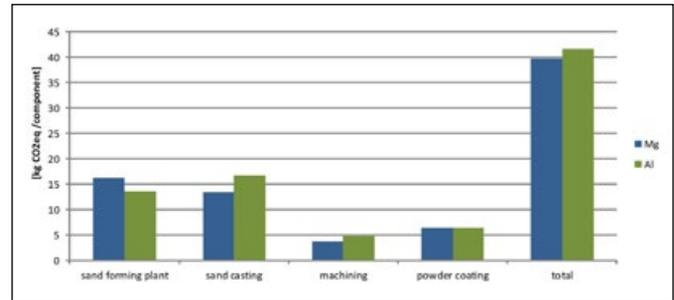
Figure 5. Contribution of the single process steps to the GHG emissions from the sand casting process.
