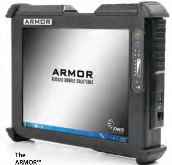
**The ARMOR™ X10mg Rugged Tablet PC has a magnesium alloy chassis and sealed fanless design that delivers all-weather functionality for rugged outdoor computing.** © Photo courtesy of DRS Tactical Systems, Inc. Used with permission.
