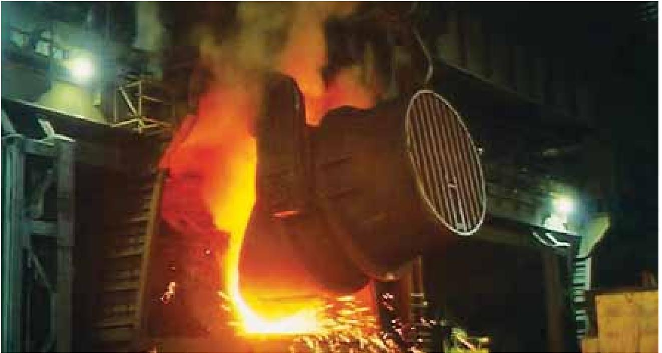
Treated metal being transferred to converter. © Photo courtesy of Almamet GmbH. Used with permission.
