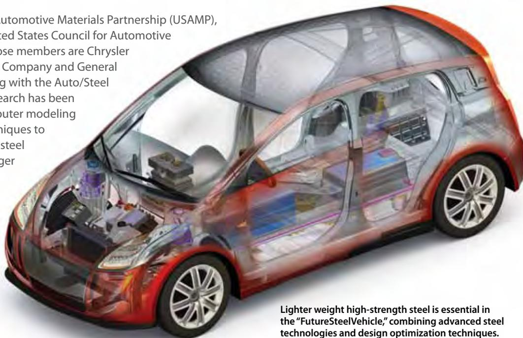
Lighter weight high-strength steel is essential in the "FutureSteelVehicle," combining advanced steel technologies and design optimization techniques. Lighter, safer structural steel parts for electrified or internal combustion engine vehicles reduce emissions over the vehicle's life cycle. © Photo courtesy of the Steel Market Development Institute. Used with permission.
