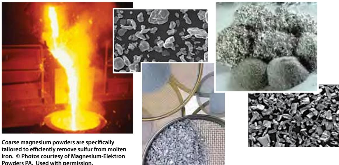
Coarse magnesium powders are specifically tailored to efficiently remove sulfur from molten iron. © Photos courtesy of Magnesium-Elektron Powders PA. Used with permission.
