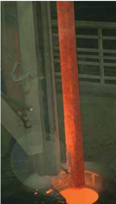
The lance is inserted into the ladle, for injection of magnesium reagent material. © Photo courtesy of Almamet GmbH. Used with permission.
