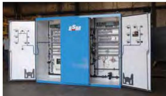
ESM's PLC continuously monitors system variables including weight, pressure and flow rate, making on-the-spot adjustments. All programming is done in-house by ESM software engineers, which results in a system that meets each customer's specific requirements. © Photo courtesy of ESM Group Inc. Used with permission.
