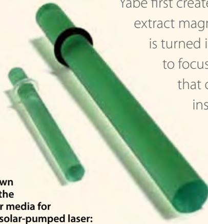
Shown are the laser media for the solar-pumped laser: the 9-millimeter diameter x 10-centimeter length used in 2008 realized 80 watts output; the 4-millimeter diameter x 5-centimeter length now realizes 70 watts output, showing vast improvement. © Photo courtesy of the Tokyo Institute of Technology. Used with permission.
