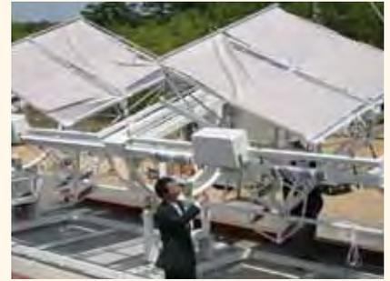
The solar-pumped laser devices build in Chitose, Hokkaido, Japan on July, 2007, producing 80W output in 2007. For safety, the 2-meter x 2-meter Fresnel lens is covered with cloth. © Photo courtesy of the Tokyo Institute of Technology. Used with permission.
