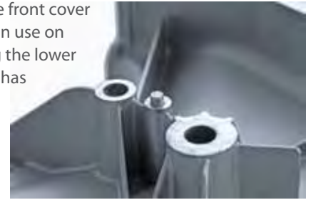
Compared to aluminum, the area tension pulley is strengthened in the magnesium cover, due to a high bending moment and compaction behavior. © Photo courtesy of Georg Fischer GmbH & Co., KG. Used with permission.
