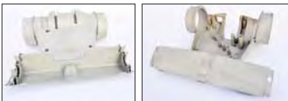
The prototype complex casting design, top view (left) creates an exotic-shaped vacuum head that lowers assembly costs and parts inventory when cast in lighter-weight magnesium, bottom view (right). © Photos courtesy of Precise Cast. Used with permission.
