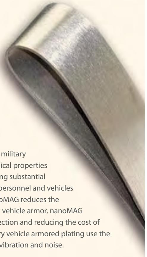
The nanoMAG process uses Thixomolded magnesium alloy for 90 percent higher strength than AZ31 sheet. © Photo courtesy of nanoMAG LLC. Used with permission.
