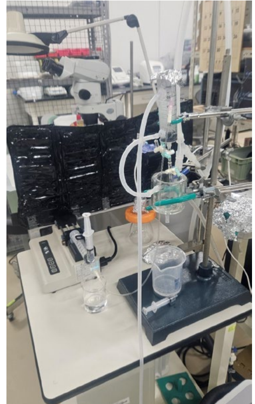
Langendorff perfusion setup in the lab.
