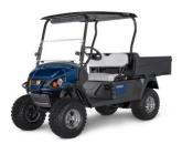
Vehicle, 72 Volt Electrical System, On Board Battery Charger, (9) 8 Volt Heavy Duty Deep Cycle Batteries, DC Converter, State of Charge Meter, 6 Ply Tires, Head, Tail & Brake Lights, Canopy Top, Fold Down Windshield, and Rear View Mirror. Lifted Suspension
