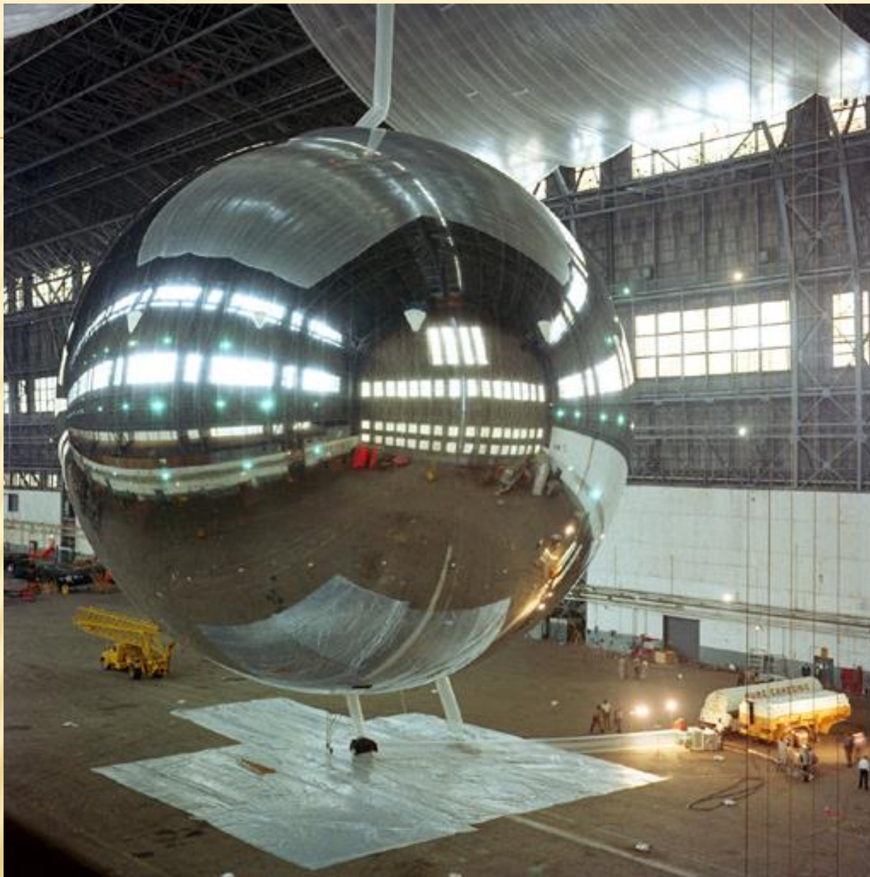
ECHO/PAGEOS BALLOON SATELLITE TYPE PHOTOGRAPHED BY BC-4
