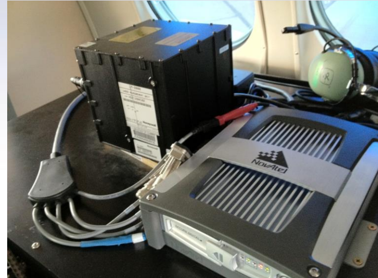
NovAtel SPAN-SE w/ Honeywell \mu IRS IMU
