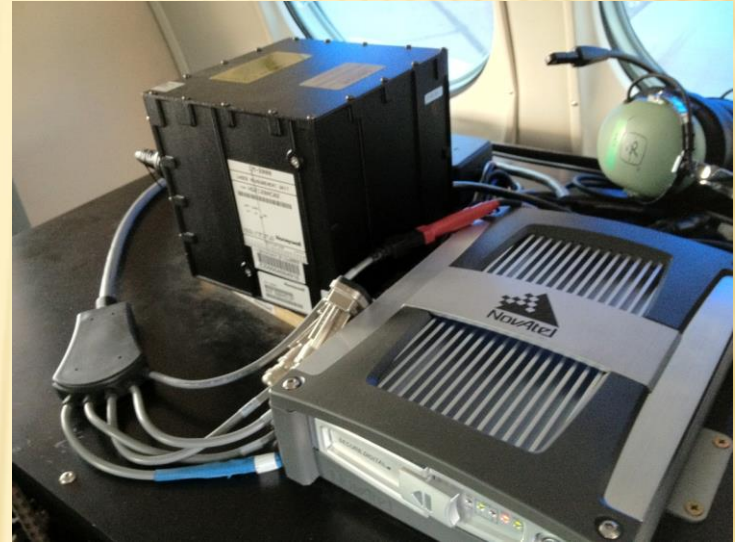
NovAtel SPAN-SE w/ Honeywell \mu IRS IMU
