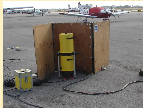
Micro-G A10 Absolute Gravity measurement
