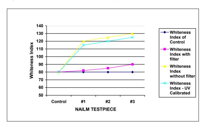
Figure: Whiteness Index of NAILM Testpiece
