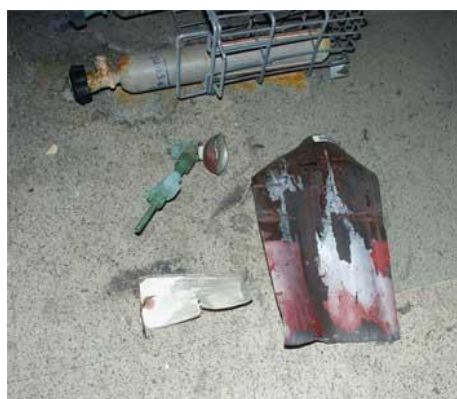
Old anhydrous hydrogen fluoride lecture bottle exploded in another university.
