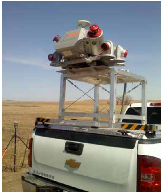
The mobile scanner offers extremely high measurement rates and provides dense, accurate, and feature-rich data at high-driving speeds.
