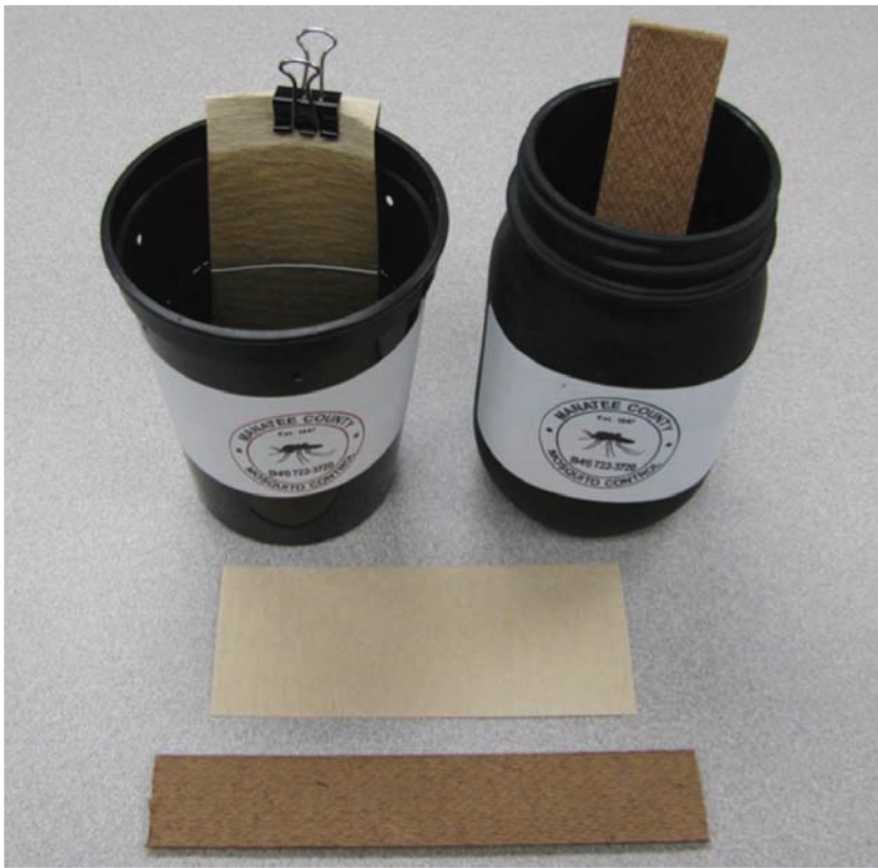
Figure 1: Ovitrap used in this study: (left) 20 oz black plastic cup with seed germination paper and (right) standard 1 pint Mason jar with masonite board.
