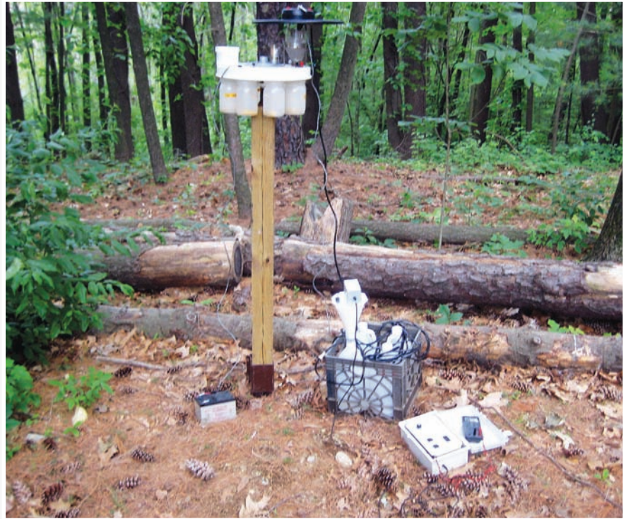
Figure 4: Blackstone CO 2 generation source baited trap setup in the field.
