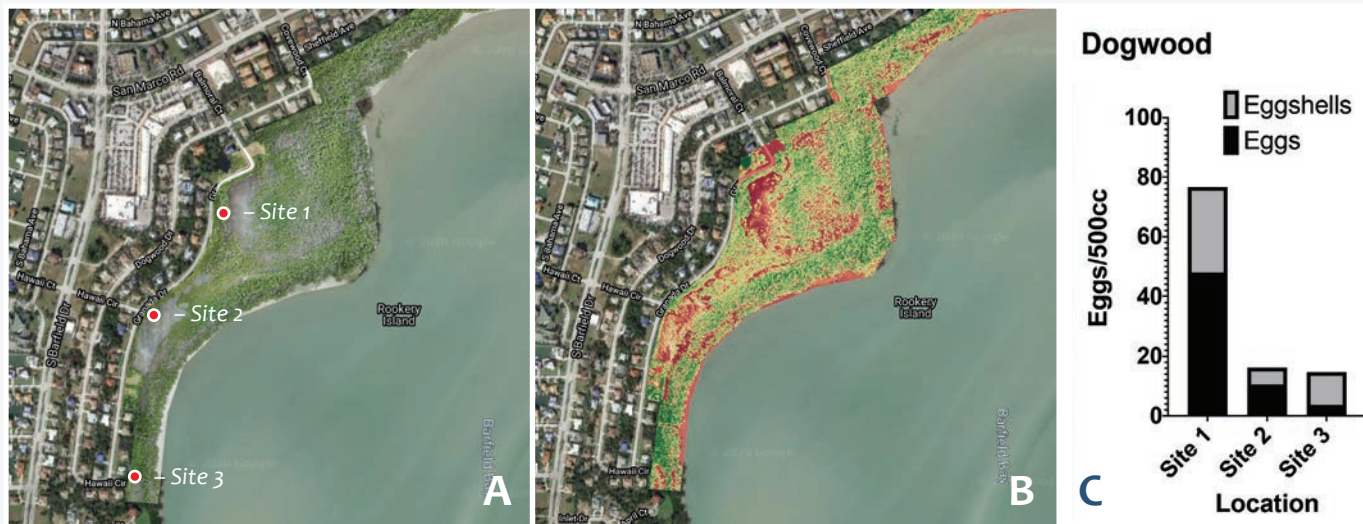
Figure 5: Identification of potential Aedes taeniorhynchus production sites using UAV technology in combination with eggshelling at the Dogwood swamp: A) Orthomosaic map; B) VARI map captured by the DJI Mavic Pro Platinum UAV; and C) Graph showing eggshell sampling results for each location.
