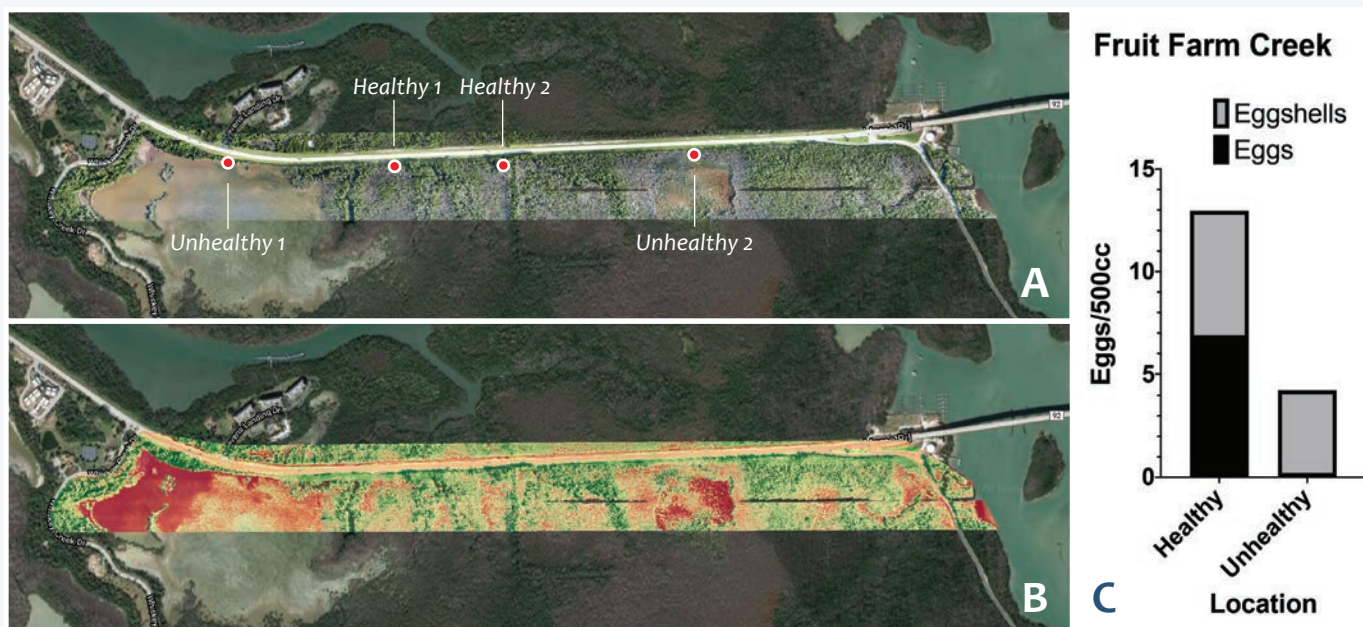
Figure 6: Identification of potential Aedes taeniorhynchus production sites using UAV technology in combination with eggshelling at Fruit Farm Creek: A) Orthomosaic map; B) VARI map captured by the DJI Mavic Pro Platinum UAV; and C) Graph showing eggshell sampling results for healthy versus unhealthy mangroves.
