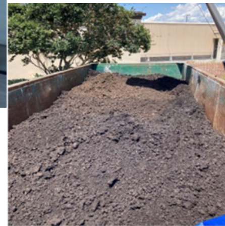
(a) TWAS gravity belt (b) Dewatering (c) Dewatered TWAS cake solids (d) Combined filtrate and wash water flowing into sump.
