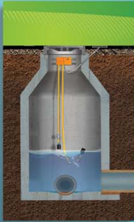
In Sewer Level Alarm
