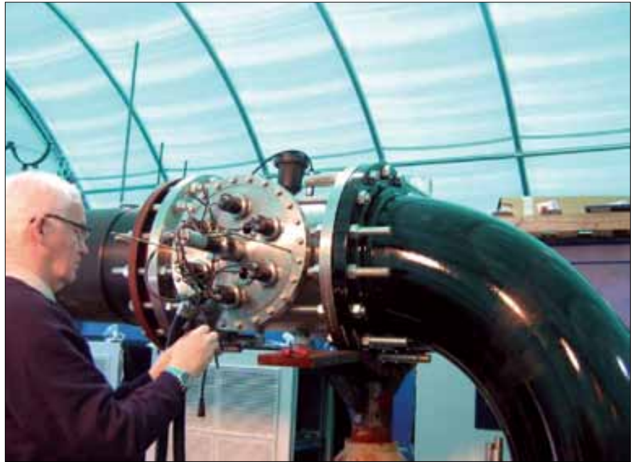
ETS lamp connections and external wiper motor
