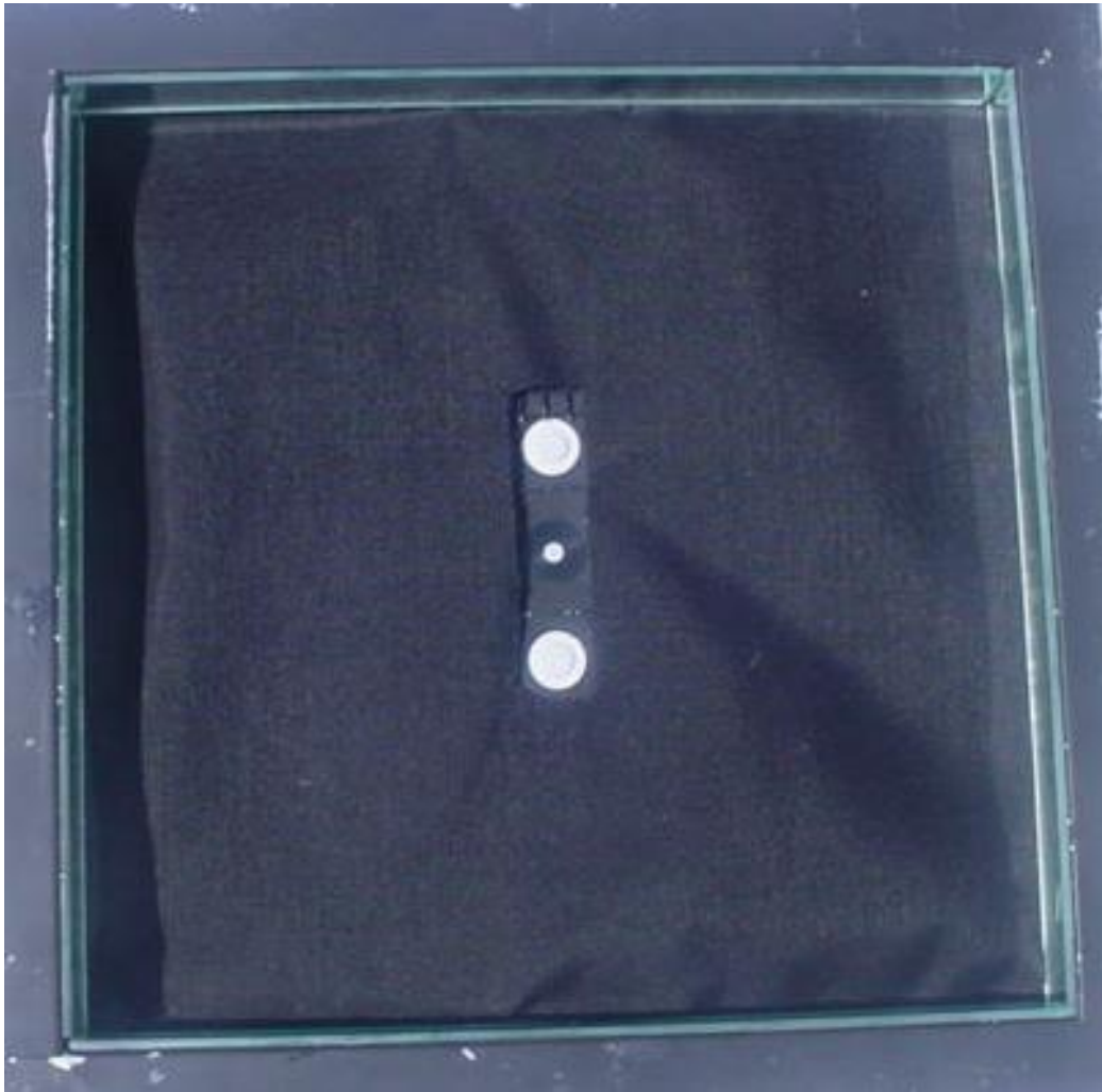
Figure A1: Photo of the test aperture. The center sensor is the photometric sensor. The other two sensors should be disregarded and removed from the apparatus for this test procedure.
