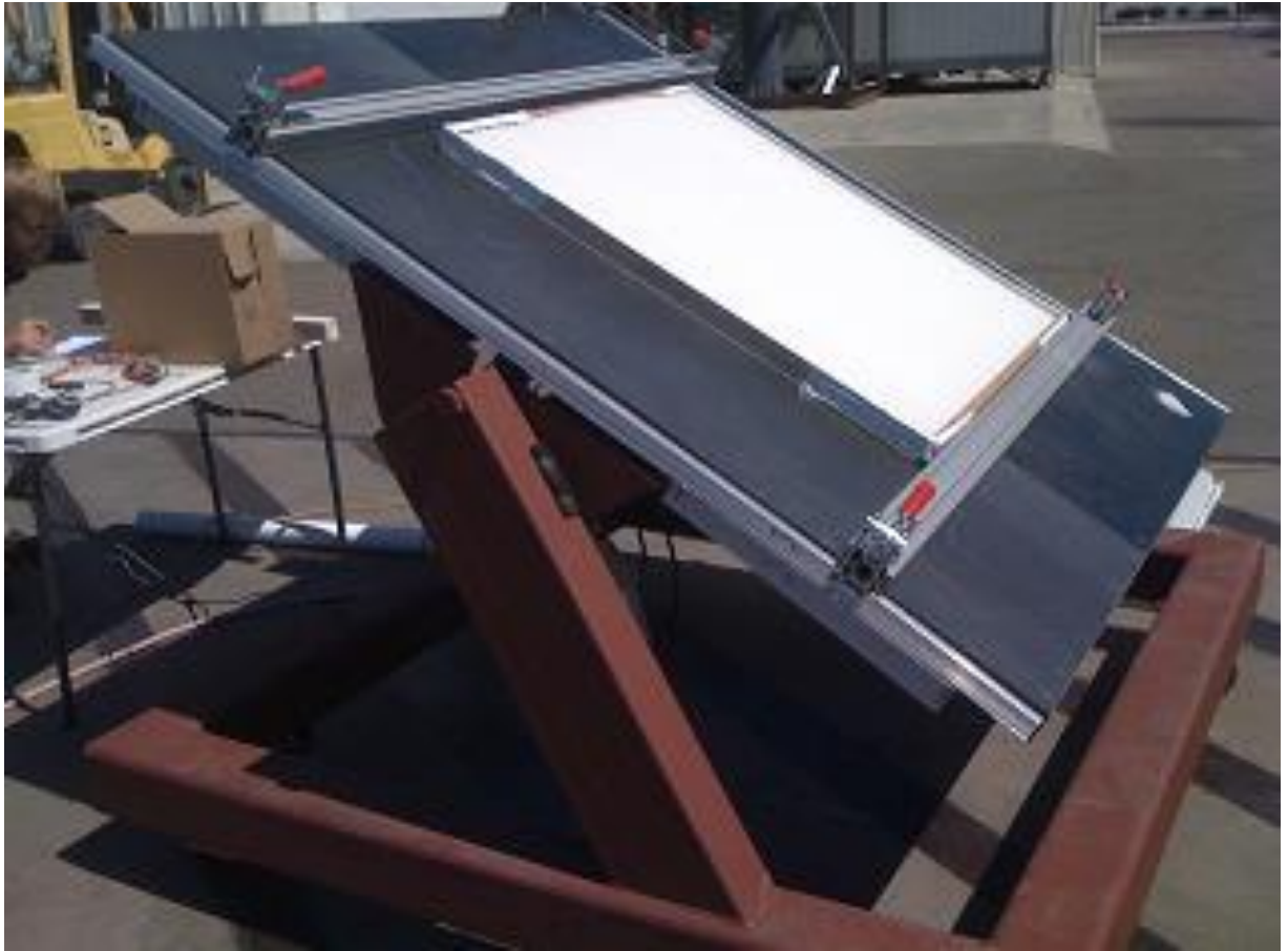
Figure A2: Photo of test apparatus with a generic test specimen centered over the aperture in the 'covered' position.
