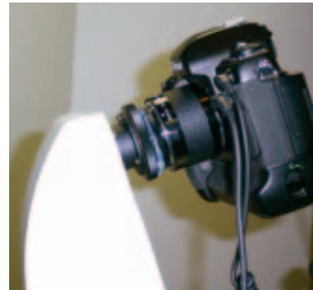
Figure 14: Topcon Relay Lens with 2x Teleconverter, Nikon D-1x camera.
