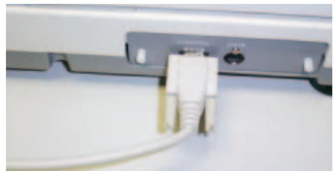
**Figure 12:** Topcon 50EX connection for digital cable.
