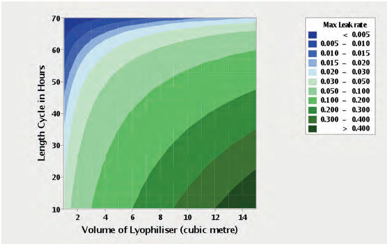
Figure 4. Visualisation of maximum leak rate in mbar L/s to ensure Grade A air quality is maintained by freeze dryer cycle and volume
