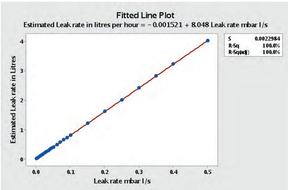
Figure 5. Estimated leak rate in litres per hour.
