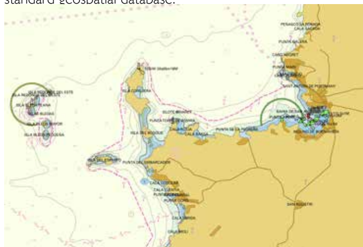
The raw S57 data dropped into our database. Note the text display, lack of small craft information, colour scheme
