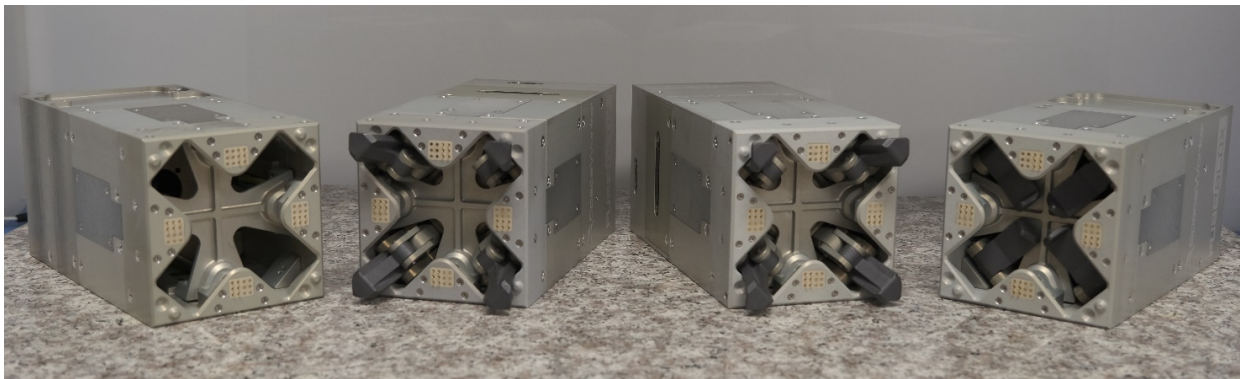
Figure 36 FuseBlox Flight Units. Left side shows an active-passive configuration, where the passive unit lacks grappling claw. Right side is showing an androgynous (active-active) configuration with left unit acting as male side
