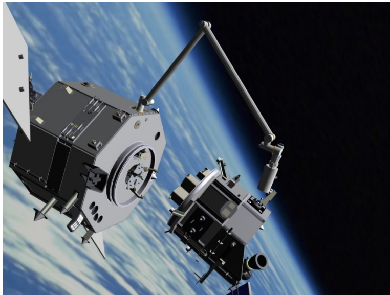
Figure 4. Robotic Arm Grappling Operation on Orbital Express
