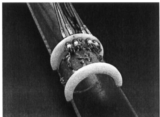
**Figure 1.** Quadrature surface receiver coil mounted on the animal holder.
