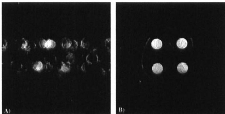
**Figure 6.** Image comparison of phantom head with four containers filled with Jell-O and a small tube filled with corn oil using an external ECG trigger (see Fig. 2, mode B). (A) Scan with ECG but without navigator gating. (B) Combined ECG and navigator gated scan, using a 2-mm acceptance window.
