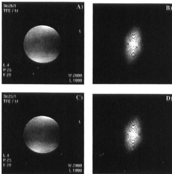
**Figure 7.** k-space yields no artifacts related to the DC motor. Image (A) and k-space (B) of a circular phantom. DC motor "off." Image (C) and k-space (D) with DC motor "on."
