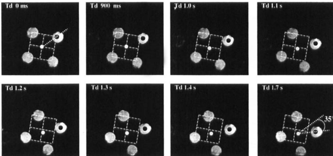
**Figure 4.** Motion phantom used in combination with its ECG (see Fig. 2, mode A). A multiple heart phase scan of the phantom head visualizes its translation and the superimposed rotation. The maximal rotation is 35 degrees (Td 1.7 sec).
