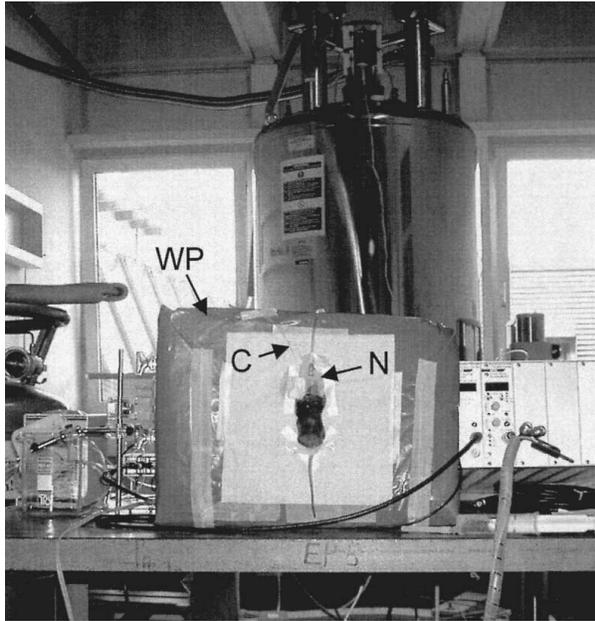
**Figure 1.** Experimental setup for in vivo measurement of LV hemodynamics with a microtip catheter. The magnet in the background is a 11.7-T vertical MR system. N, nose cone for isoflurane anesthesia; C, catheter lead connected to the pressure transducer; WP, warming pad.
