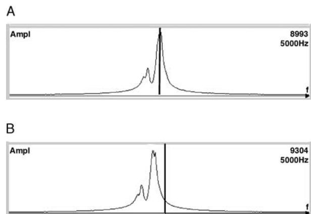
**Figure 8.** Representative display of fat (left peak) and water (right peak) frequency spectrums. The baseline automatic frequency option was 63.661808 MHz (A). The vertical black line, at 63.662009 MHz, shows representative position manually chosen to create the off-frequency tuning error artifact shown in Fig. 7B (B).
