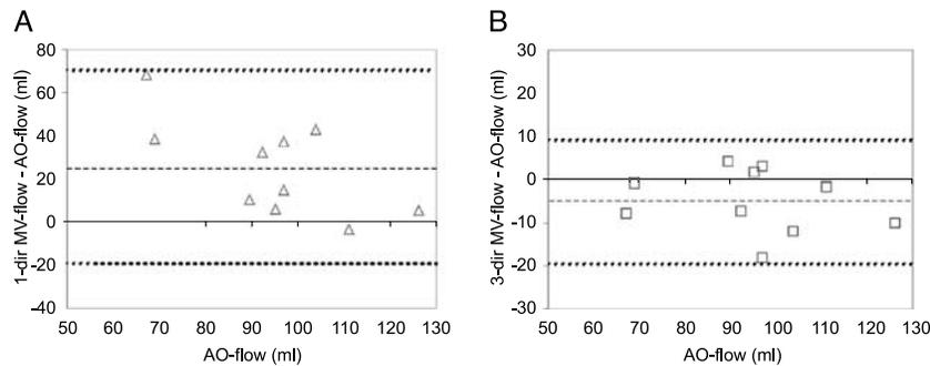
**Figure 4.** Bland-Altman analysis for studying the differences between the MV-flow volume [determined with the 1-dir MV-flow method (A) and the 3-dir MV-flow method (B), respectively] and the AO flow. The 1-dir MV flow shows a statistically significant overestimation compared to the AO flow. The 3-dir MV flow is not statistically significantly different. The dashed lines represent the mean differences, the dotted line determines the 95% confidence intervals.
