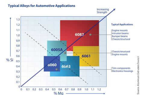
Design engineers have a variety of alloy options for making extruded aluminum auto components. Typical applications for trucks and cars include engine mounts, intrusion beams, bumper beams, chassis and structural components, trim, and electronics housings.
