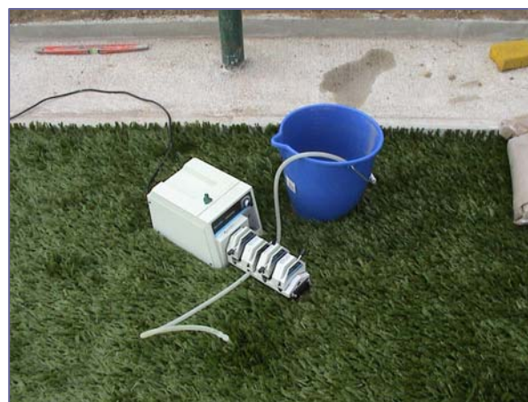
Figure 5: System for the recovery of the percolates collected in the lysimeter situated under the artificial turf by means of a pipe crossing the artificial turf and connected to a sampling pump.
