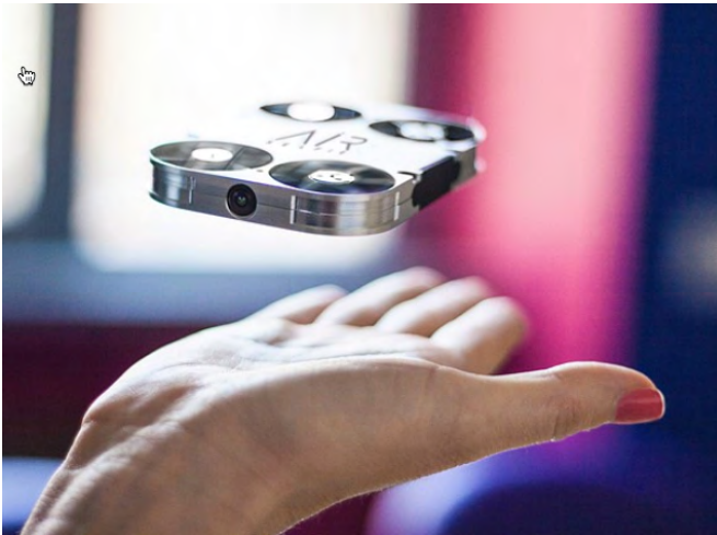
Figure 1 The Air Selfie –when you want an aerial selfie, you slip this out of your phone case, quickly assemble it and using a phone app, fly it over your group for an aerial selfie.
