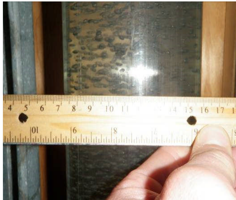
Course Bubble Aeration
