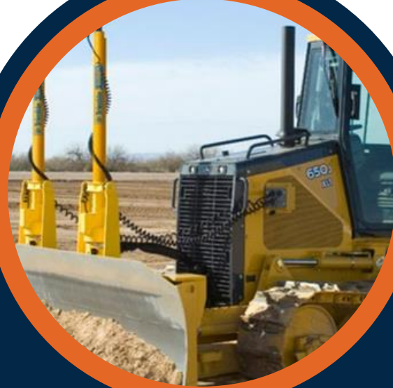
2D LASER GRADING
