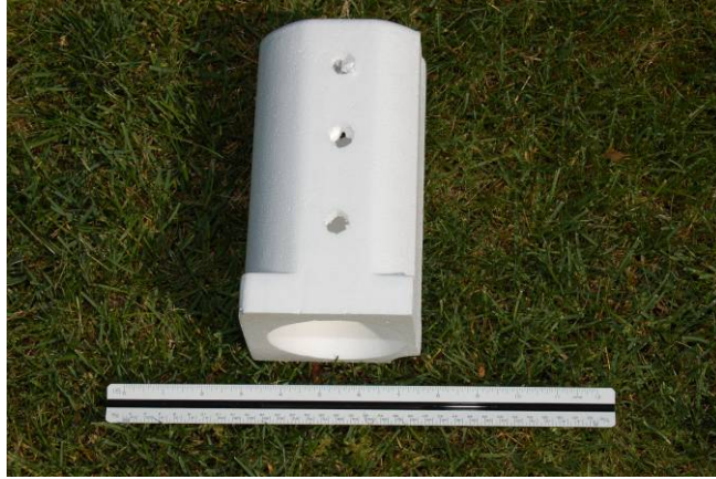
Figure 2 - Styrofoam cylinders used for temperature measurements
