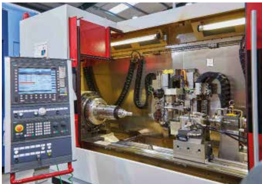
This Kapp Niles VX-series, 90-degree profile grinding machine allows for sequential roughing and finishing tool use
