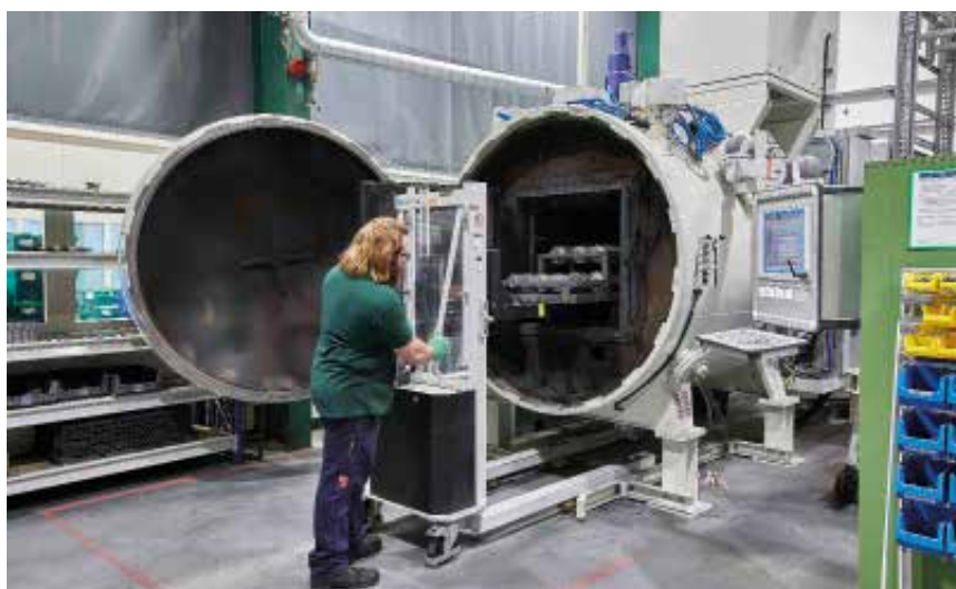
Heat treatment of parts is all done in-house, and is gradually moving towards the low pressure carburising solution
