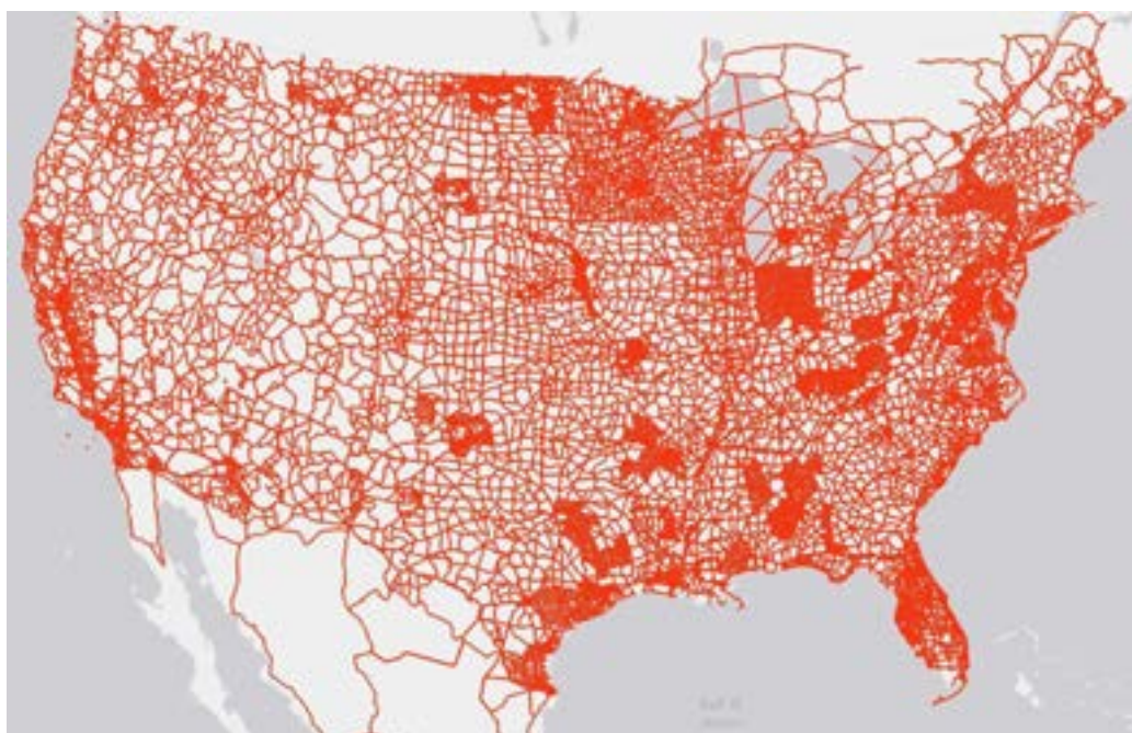
Figure Geodetic-1. Partial vertical control network used in NAVD 88. Additional lines run through Canada to Alaska, but NAVD 88 is an authoritative vertical datum only in the Conterminous U.S. and Alaska. Source: NOAA.
