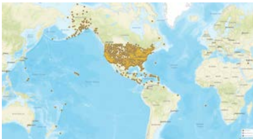
Figure Geodetic-3. NOAA CORS Network provides nearly 2000 active control stations for access to the NSRS. Source: NGS, 2024 ( https://geodesy.noaa.gov/CORS/ for info and https://arcg.is/18fWq8 for data).
