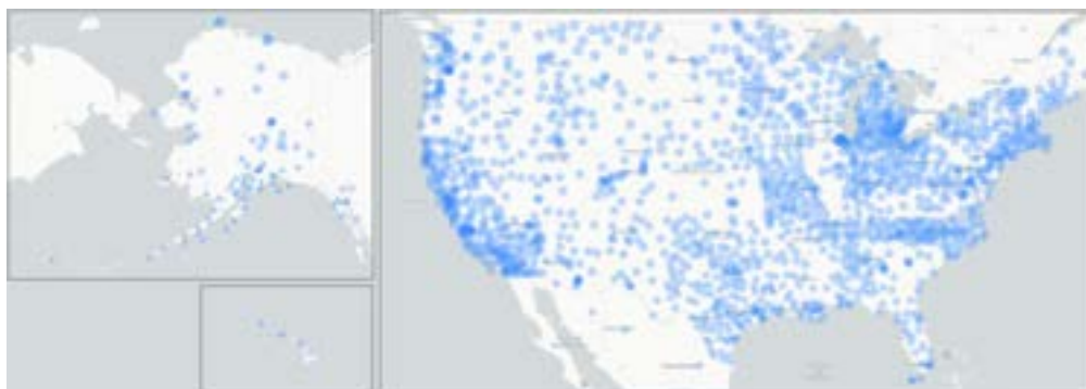
Figure Geodetic-10. Coverage extending 35 kilometers around Operational CORS in the United States, as of March 8, 2024. Source: NOAA.
