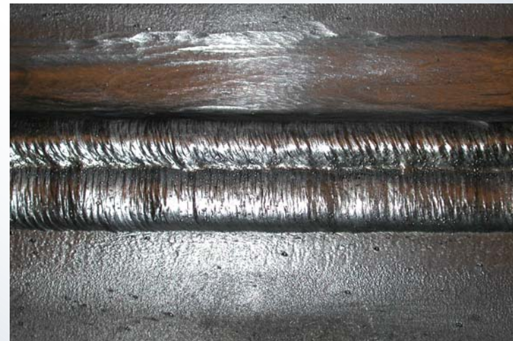
Ti-CP Weldment Produced with Double Pulse/Droplet Waveform
