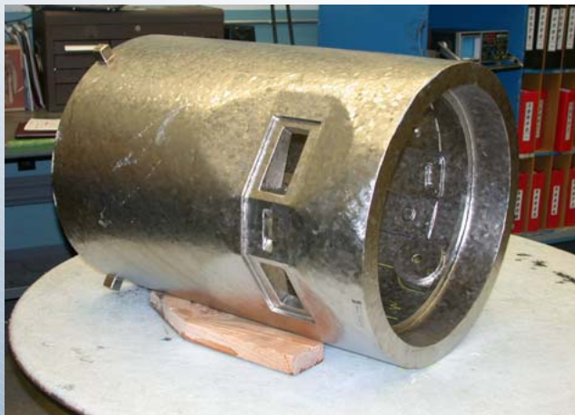
Trial Casting Ti CP-2LO UUV Hull Section
