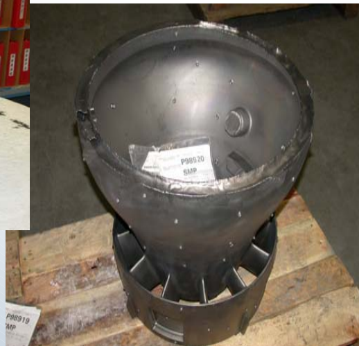
Trial Casting Ti-5111 UUV Hull Section
