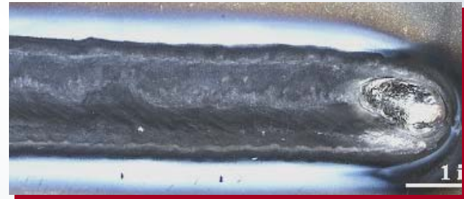
GTAW with Ti CP-2 flux-cored wire
