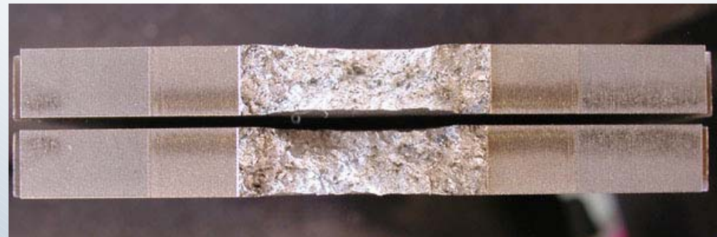
← Cast Ti CP-2 1-in Thick
