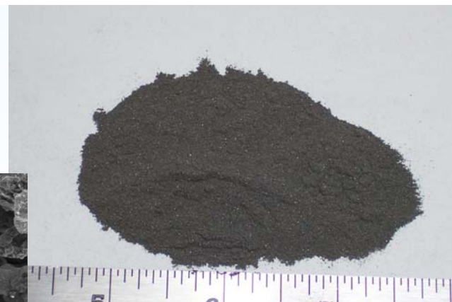
TiH 2 powder (-100 mesh) grinded at ADMA Products, Inc.
