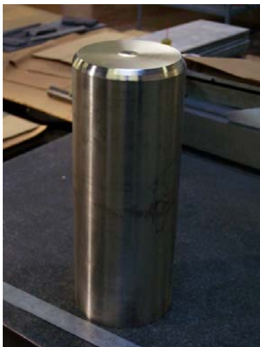
P/M Ti-6Al-4V Extrusion billets
