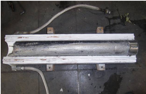
Figure 5: VIM-cast TiAl electrode ( \varnothing 105 mm, L 750 mm, mass approx. 25 kg)
