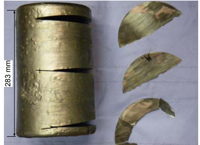
Figure 7: Sampling of obtained, deoxidized PESR ingots
