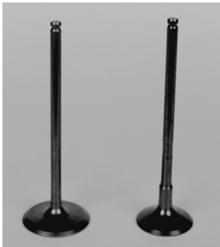
Figure 6. The developed BE titanium intake valve (left) and Ti-MMC exhaust valve (right).
