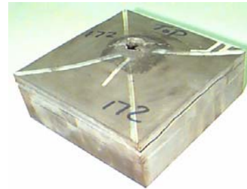
Figure 17. Hot Isostatically Pressed Ceramic in Titanium Matrices
