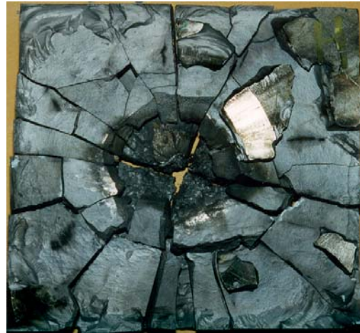
Figure 16. Functionally Graded Titanium Monoboride/Titanium Plate
