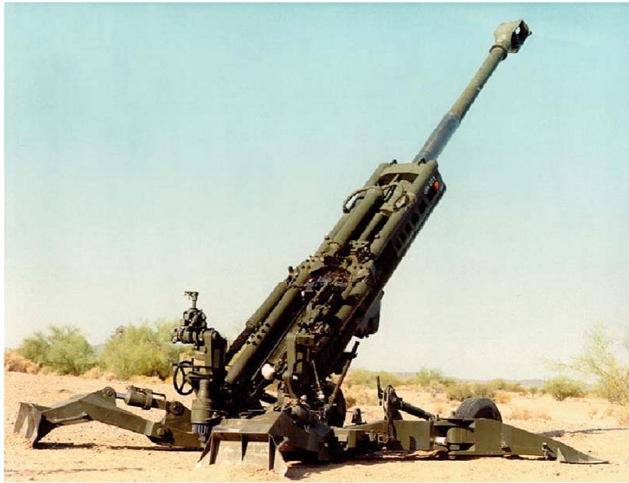
Figure 21. Ultra-light Weight M777A1 Towed Howitzer Utilizes Extensive Titanium Castings
