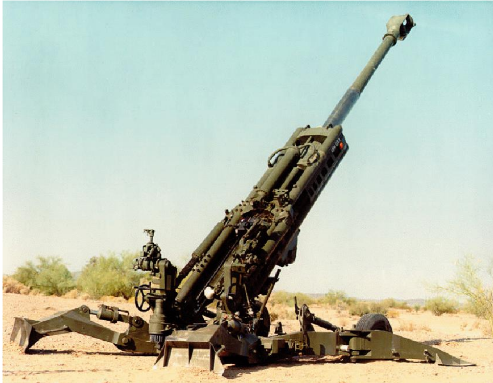
Figure 21. Ultra-light Weight M777A1 Towed Howitzer Utilizes Extensive Titanium
