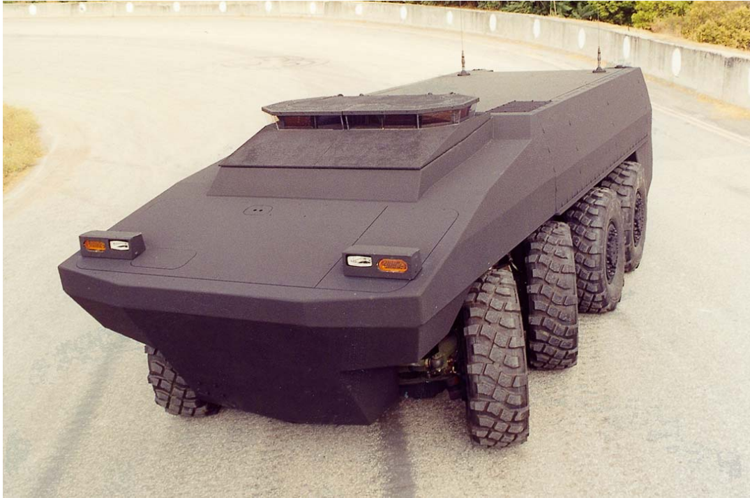
Figure 22. BAE Pegasus Titanium Wheeled Prototype
