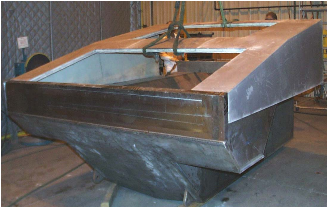
Figure 23. Future Combat Vehicle Titanium Hull Prototype
