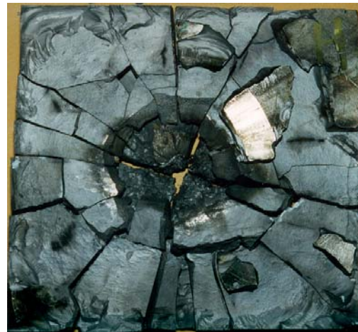
Figure 16. Functionally Graded Titanium Monoboride/Titanium Plate
