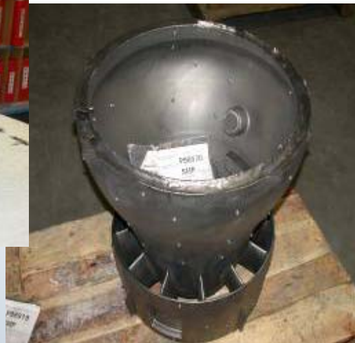
Trial Casting Ti-5111 UUV Hull Section
