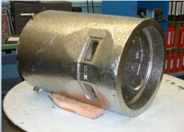
Trial Casting Ti CP-2LO UUV Hull Section
